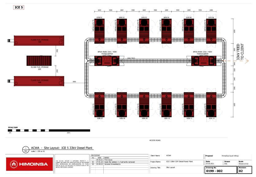
Figure 2-3: Proposed site layout for ICE 5
