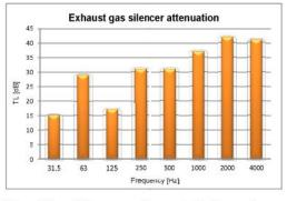
Figure 12. Exhaust gas silencer typical transmission loss
