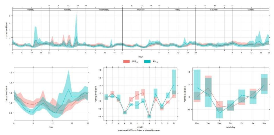
Figure 5-7: Diurnal and seasonal variation plots of observed PM<sub>2.5</sub> and PM<sub>10</sub> at the DFFE Karoo AQMS (shaded area indicates 95<sup>th</sup> percentile confidence interval)
