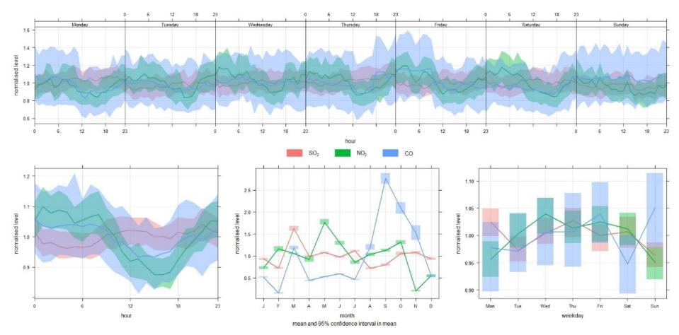
Figure 5-6: Diurnal and seasonal variation plots of observed SO<sub>2</sub>, NO<sub>2</sub>, and CO at the DFFE Karoo AQMS (shaded area indicates 95<sup>th</sup> percentile confidence interval)
