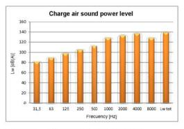
Figure 13. Charge air sound power levels
