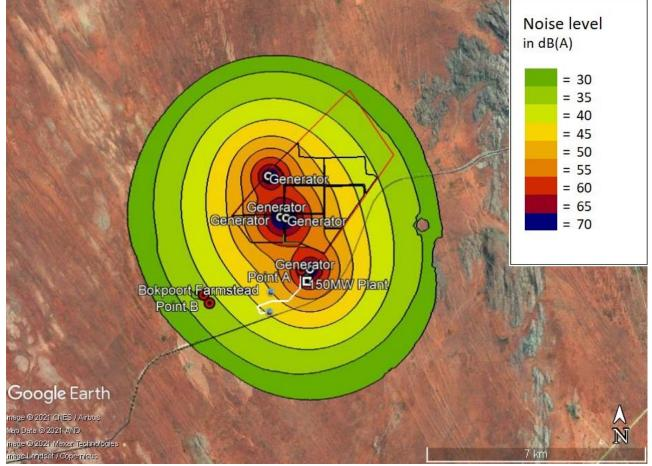
Figure 7-3: Predicted Noise Contour Map of the Cumulative Operational Phase of both Proposed Projects
