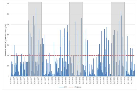
Figure 5-13: Simulated time series of ambient NO<sub>2</sub> concentrations at the closest receptor assuming continuous operation for the purposes of identifying suitable periods for the reliability tests (grey blocks indicate the highest number of exceedances of the NO<sub>2</sub> NAAQ limit concentration)
