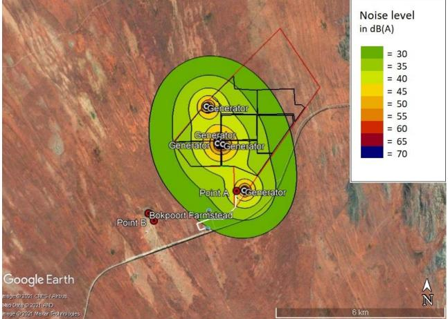
Figure 7-1: Predicted Noise Contour Map of the Construction Phase
