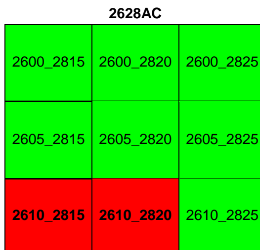
Figure 3: The 2628AC q.d.g.c. (15 minutes of latitude by 15 minutes of longitude, 15' x 15') is divided in nine smaller grids (5 minutes of latitude by 5 minutes of longitude, 5' x 5') of which each represent a pentad. The pentads in red represent the pentads in which the study area is situated.
