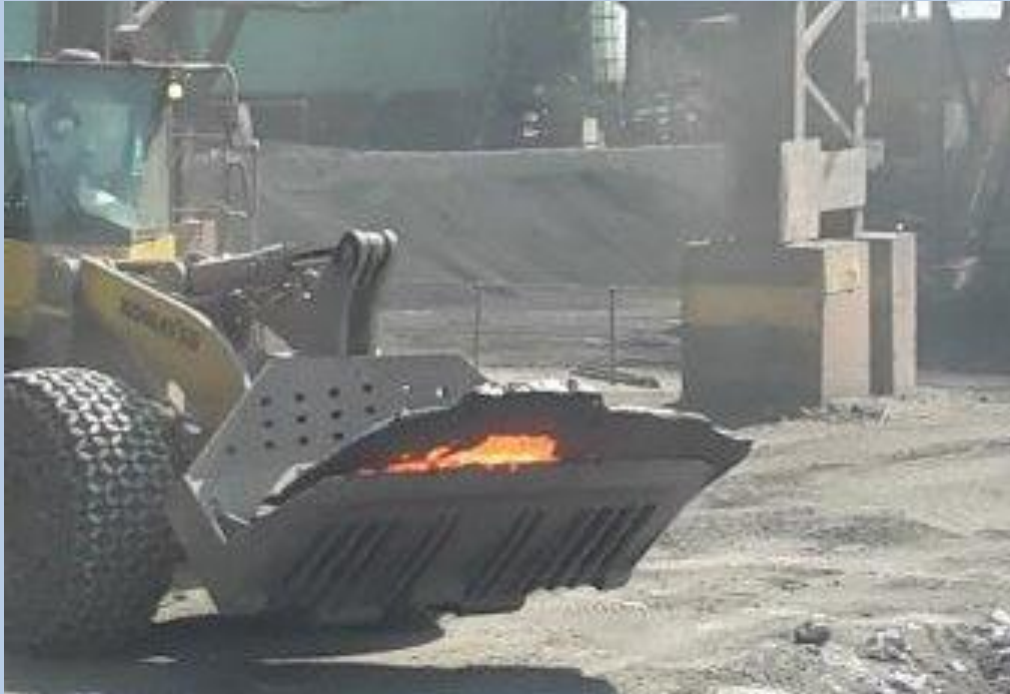
Figure 2: Chrome Slag being removed from the smelting process
