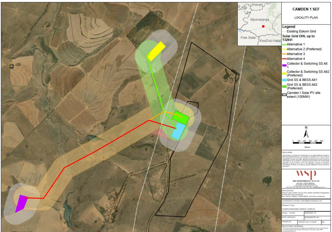
Figure 1-2: Locality map for the proposed Camden I SEF up to 132kV OHPL project, showing the respective grid route corridors and assessment zones around the substation infrastructure.
