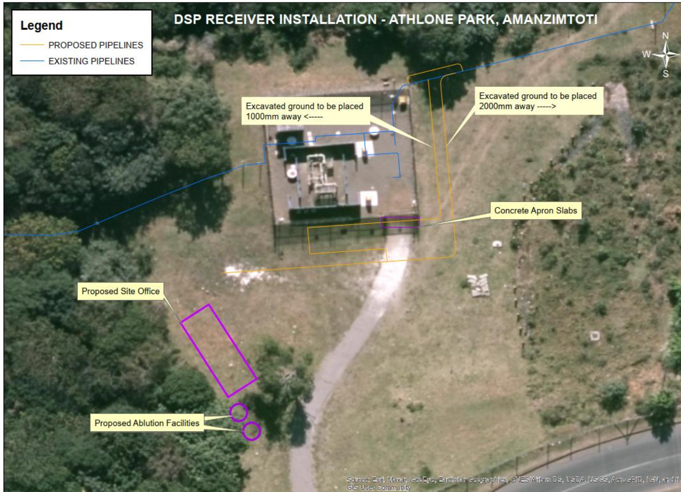
Figure 3-1 – Sasol PRS and the proposed structures and pipeline associated with the Receiver Station (to be constructed on apron slabs)
