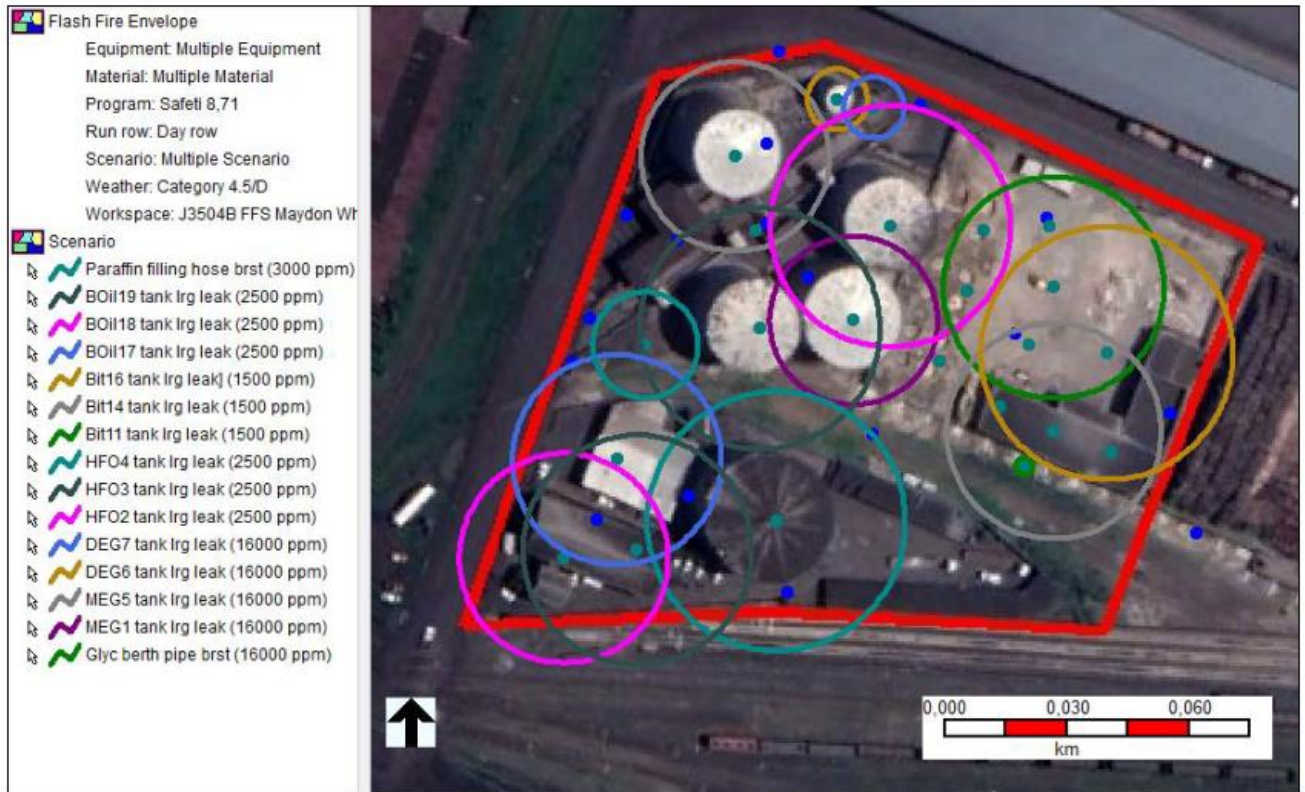
Figure 8-17 - Radiation circles for half the Lower Flammable Limit (0.5 LFL), the MHI threshold (Class 3 Materials – Worst Cases)
