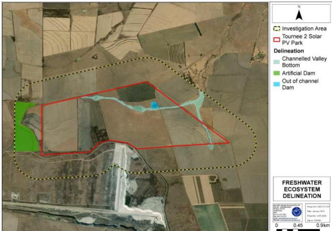
Figure 6-9 - Freshwater ecosystem delineations (field-verified) associated with the proposed Tournée 2 Solar PV Park
