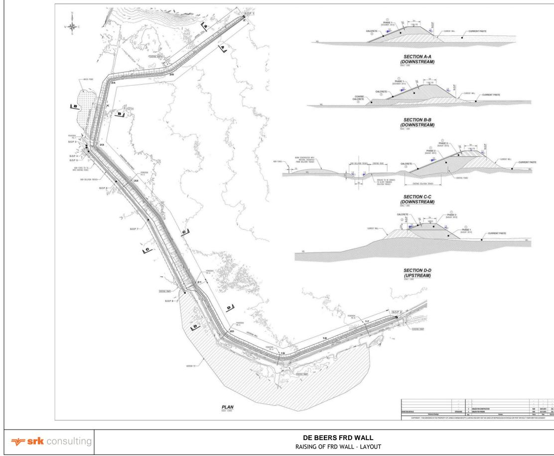
Figure 1: Engineering Design for Raising the FRD Wall
