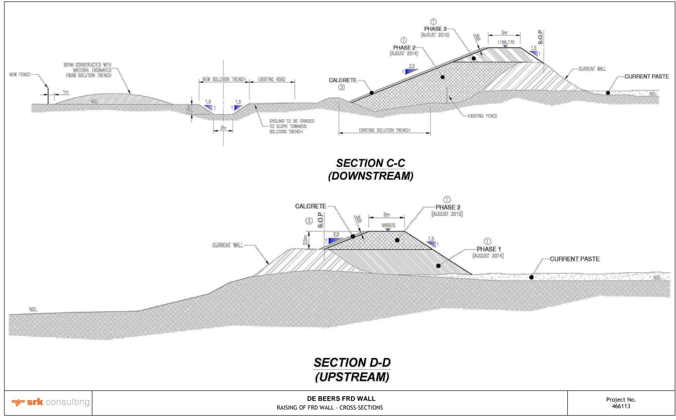
**Figure 2:** Typical Downstream (Exterior) and Upstream (Interior) Cross-sections Source: Jones and Wagener, 2013
