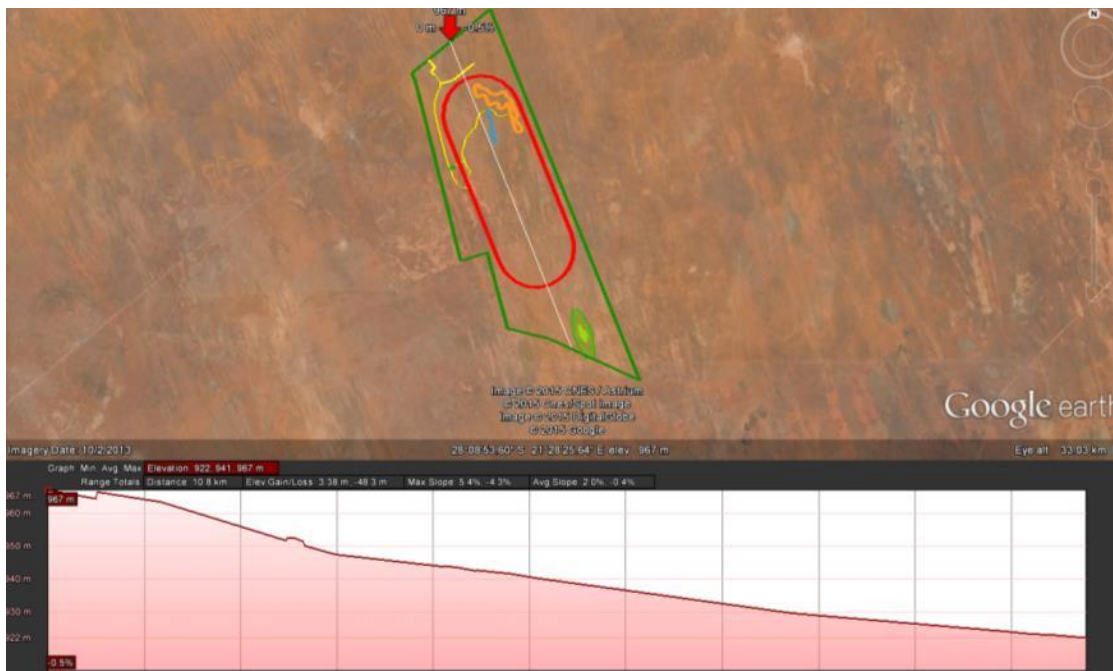
Figure 7-4: Elevation Data Shows a Slight drop in elevation from North to South and East to West
