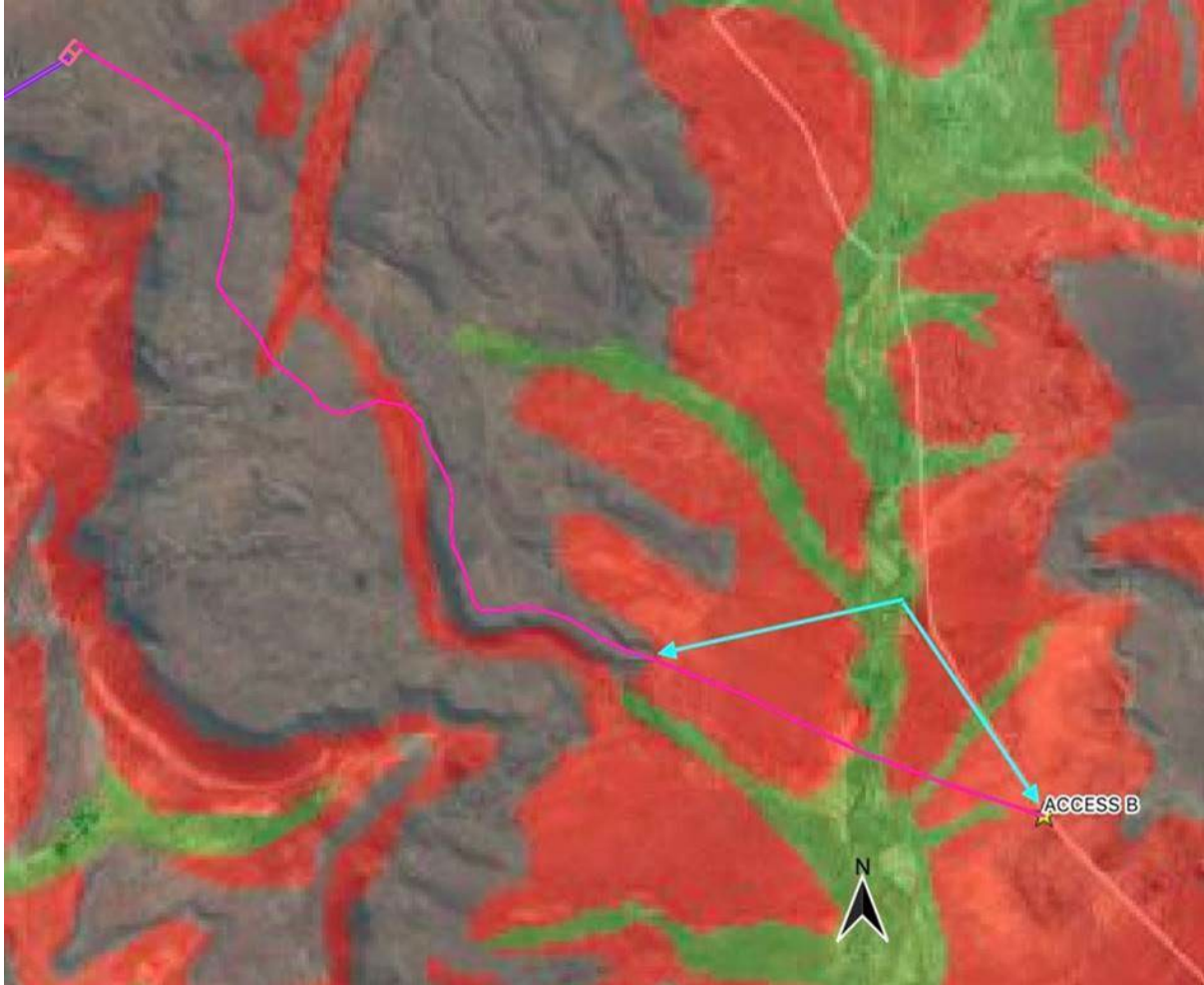
Plate 1: Proposed Access Road overlain by the paleo sensitivity. Light blue marker highlights a section of the proposed access road (pink line) which crosses an area of palaeontological sensitivity (approximately 4 km).
