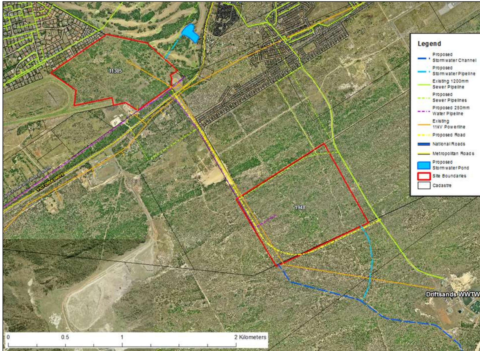
Figure 2-2: Conceptual drawing showing existing and proposed bulk service connection alignments for the development
