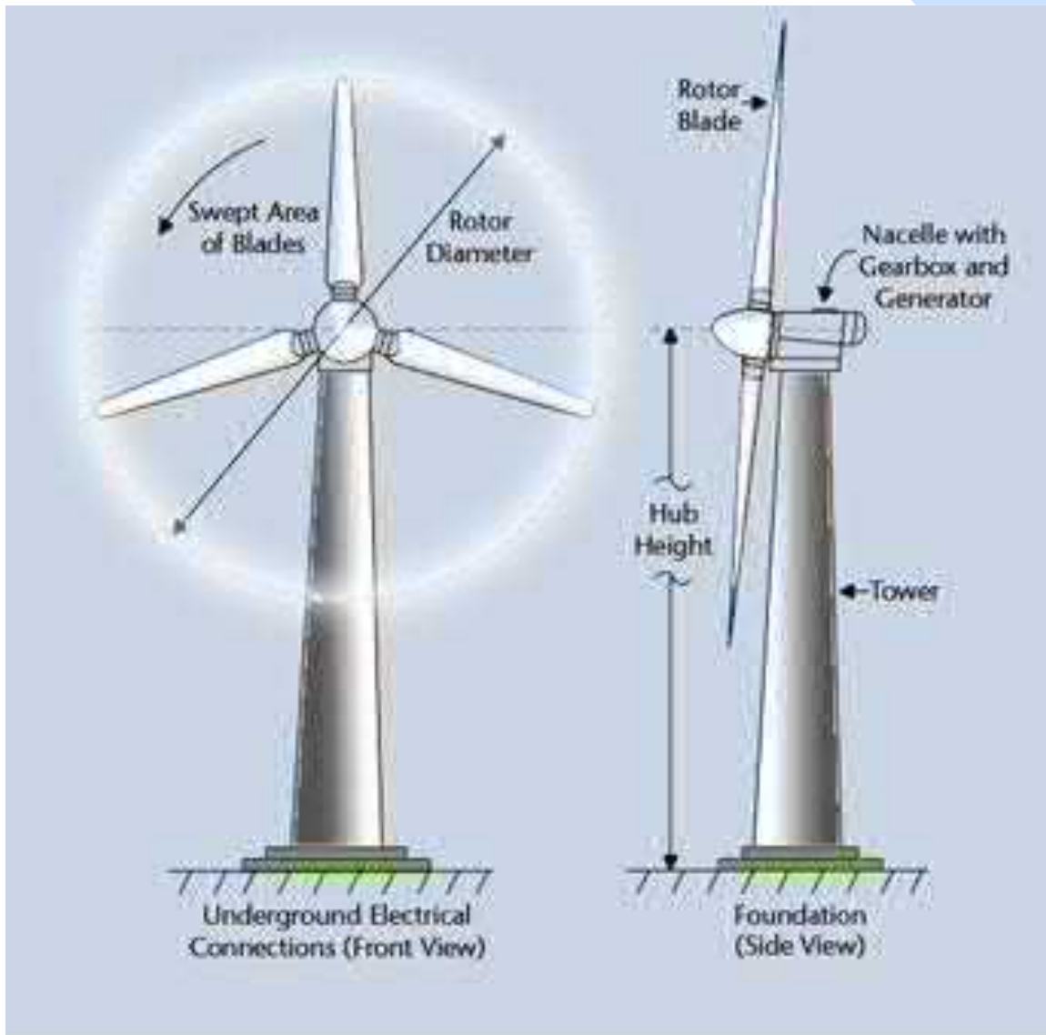
Drawing of the rotor and blades of a wind turbine, courtesy of ESN
