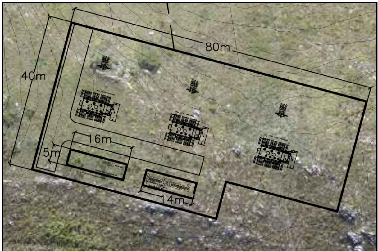
Figure 2-10: Electrical substation preliminary design (see Appendix F for larger drawing) (Source: Africoast)
