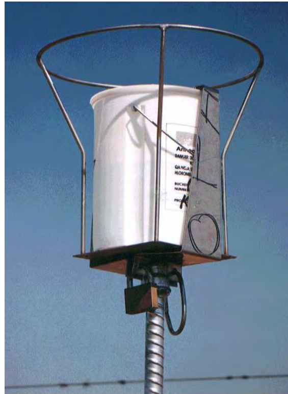
Figure 1: Single bucket monitoring unit, showing a sampling bucket with bird ring and security clamp.
