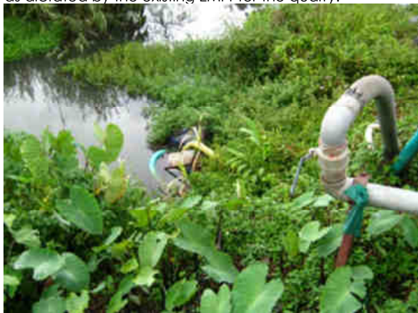
Photo 16. View of the current water abstraction pump placed within the Vungu River channel and being operated by the quarry to facilitate dust suppression on the plant (mechanical) equipment.
