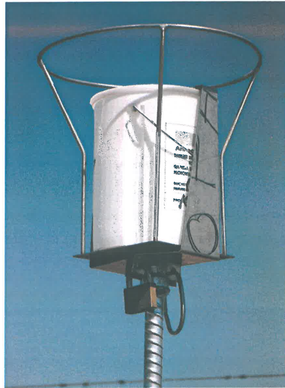
Figure 1: Single bucket monitoring unit, showing a sampling bucket with bird ring and security clamp.
