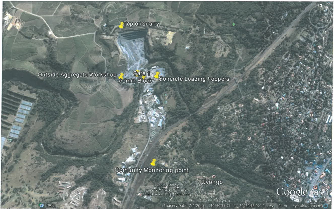
Figure A2.1: Map illustrating the location of the bucket monitoring sites at South Coast Stone Crushers
