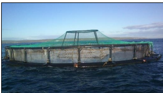
High density polyethylene (HDPE) fish cage moored in Big Bay, Saldanha Bay
