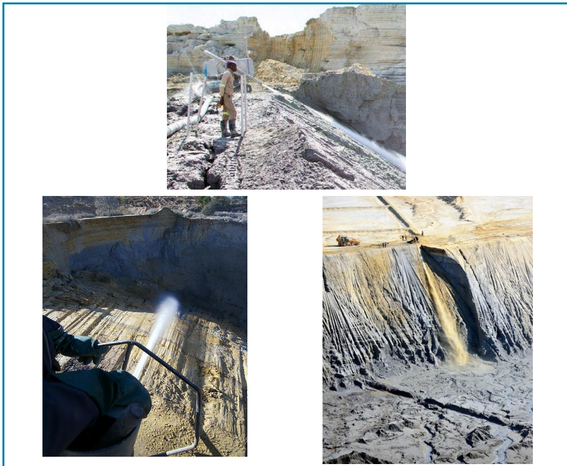
Figure 2: Mobile tracked hydraulic monitor on a tailing's facility in South Africa.
