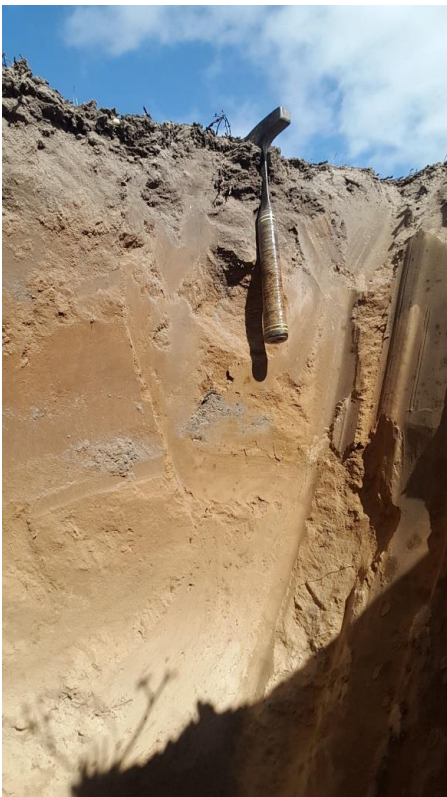
Figure 5. Photographs showing typical soil profiles from the site. Left is a deep sand of the Witfontein soil form. Right is a soil of the Glencoe soil form with a hard plinthic B horizon in the subsoil.
