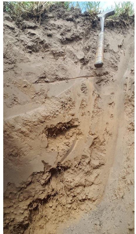
Figure 5. Photographs showing typical soil profiles from the site. Left is a deep sand of the Witfontein soil form. Right is a soil of the Glencoe soil form with a hard plinthic B horizon in the subsoil.
