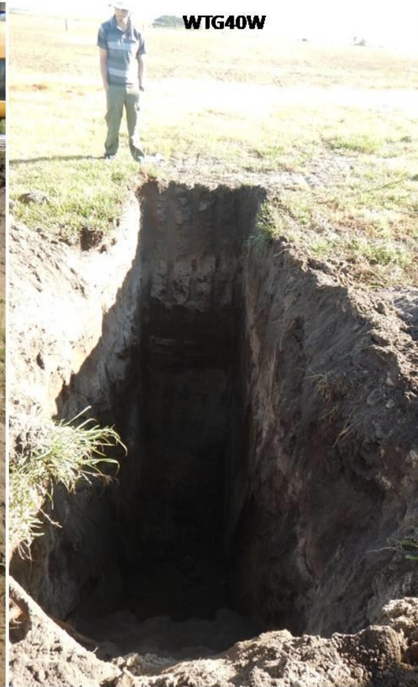
Plate 17. Geotechnical test pits at WTG39, 40 and 41W. Excavations are between 4 and 5 m deep. No archaeological traces or anthropogenic layers were seen.
