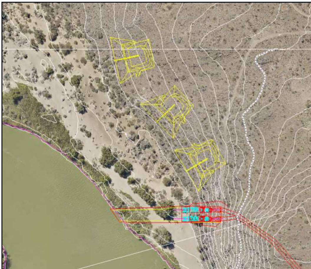
Figure A3.1: Aerial photograph with the three proposed silt storage areas indicated in yellow.
