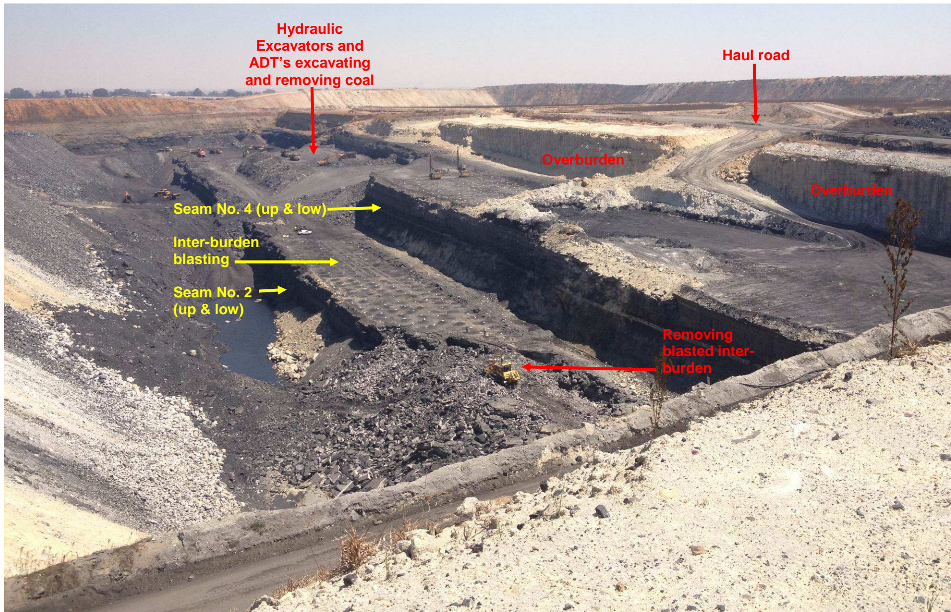
Figure 4: Opencast Coal Mining Process (Vlakfontein Central Block)
