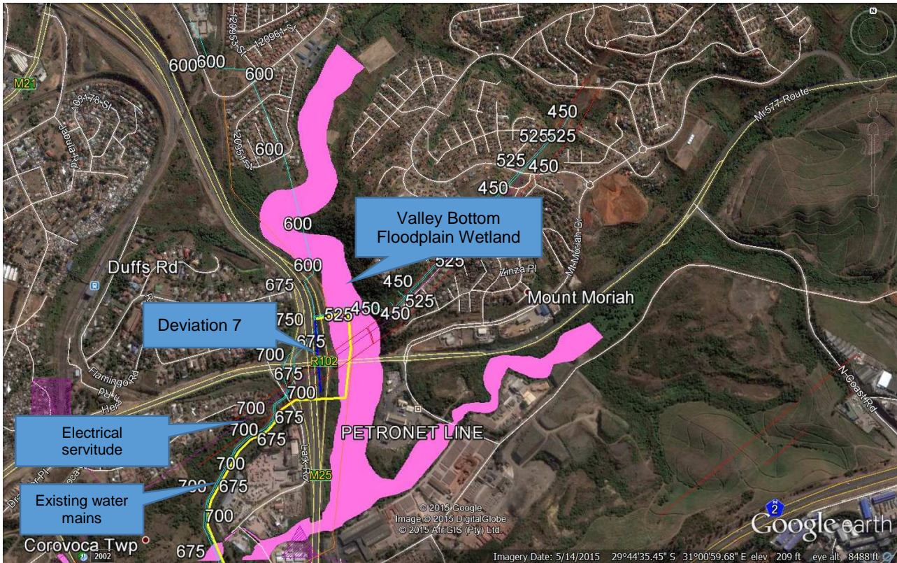
Figure 8: Deviation 7 Deviation 7: Blue line avoids encroachment into the Valley Bottom Floodplain Wetland Yellow line is the original pipeline route
