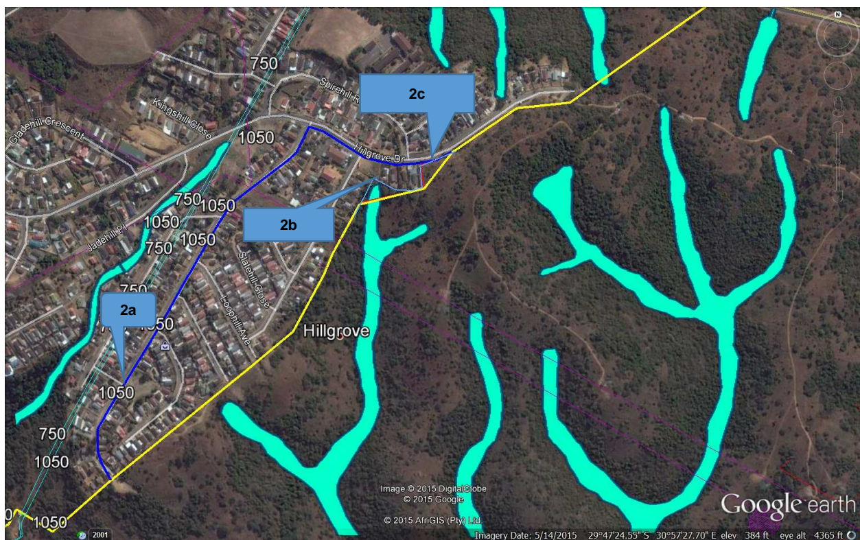
Figure 3: Deviation 2a, 2b and 2c Deviation 2a: Blue line is the suggested deviation along Royalhill Road Deviation 2b: Light blue line follows the edge of the cadastral boundary Deviation 2c: Light blue line follows along Hillgrove Drive The yellow line is the original preferred pipeline route
