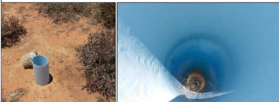
Figure 38: Dry hydrocensus boreholes showing casing and cap and down borehole photos
