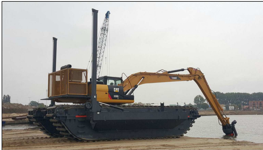
Figure 9: Example of an excavator and slurry pump potentially to be used by MSR on the beaches
