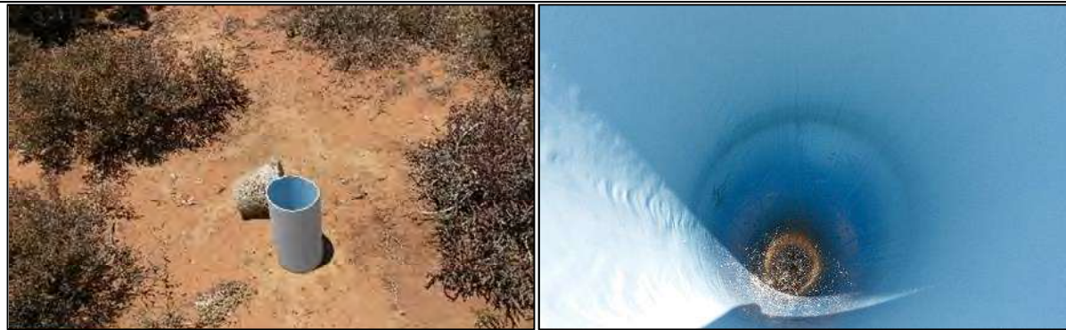
Figure 35: Dry hydrocensus boreholes showing casing and cap and down borehole photos
