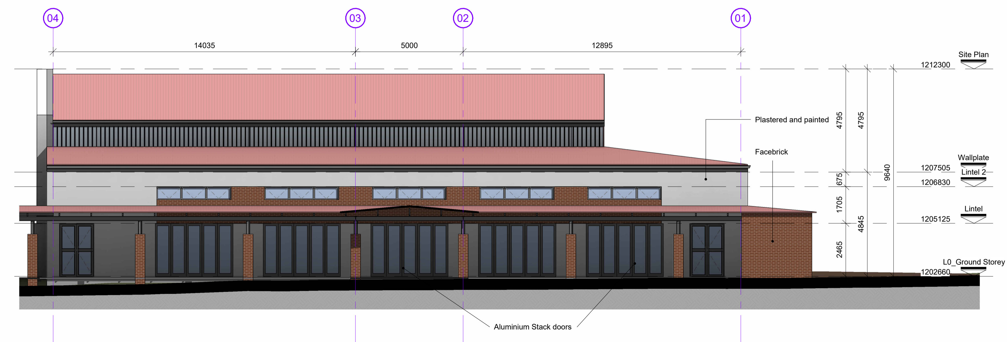
North West Elevation 1 : 100
