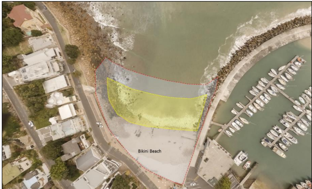
Figure 3-4: Bikini Beach historic profile (red dashed line) and expected profile after depositing of dredged sand (yellow area)
