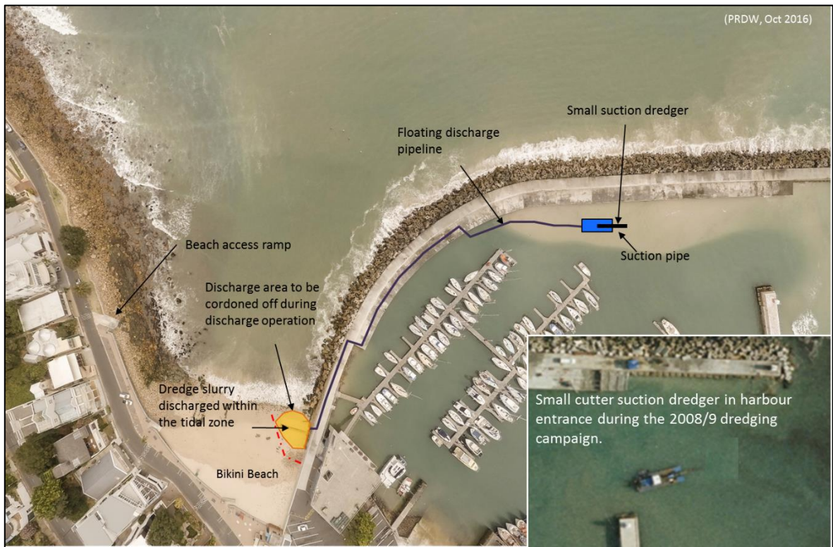
Figure 1-3: Proposed maintenance dredging operation and dredge material discharge
