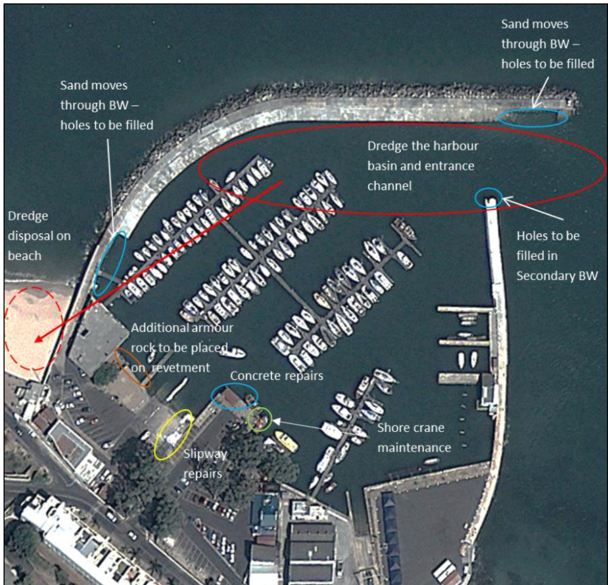
Figure 3-1: Repair and maintenance work required at Gordon's Bay Harbour
