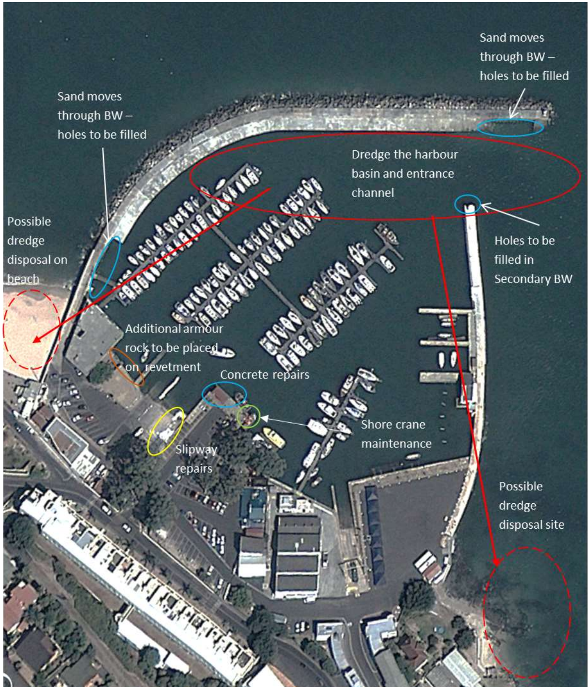
Figure 2-2: Work required in Gordons Bay Harbour
