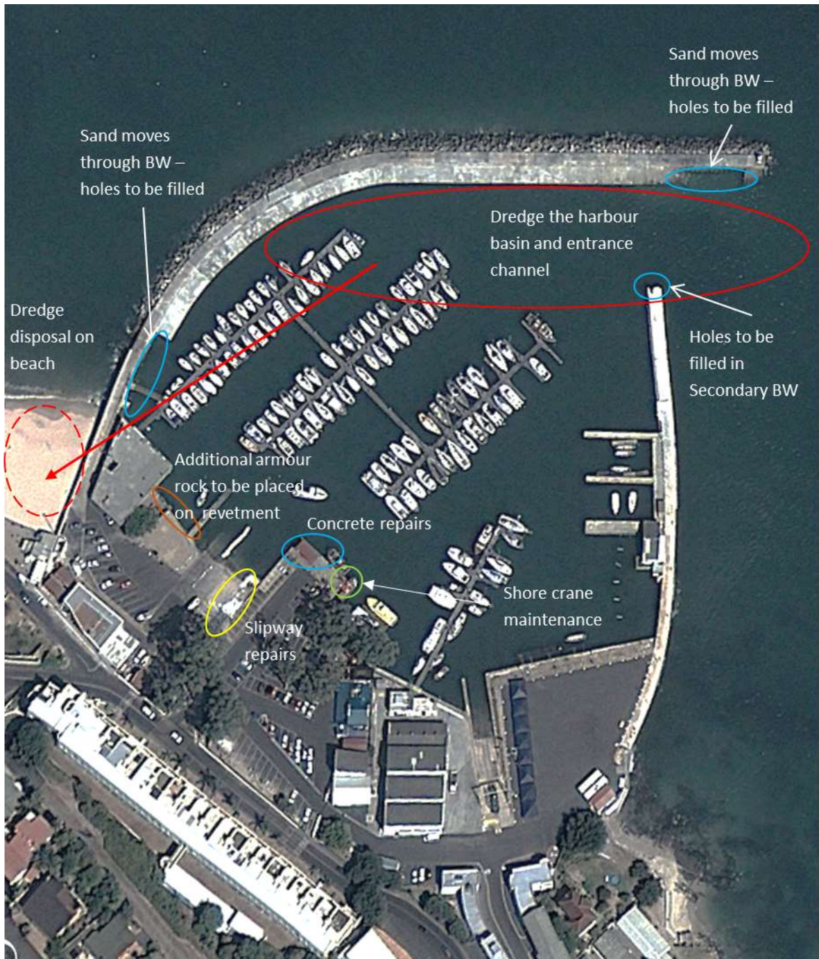
Figure 2-2: Work required in Gordons Bay Harbour
