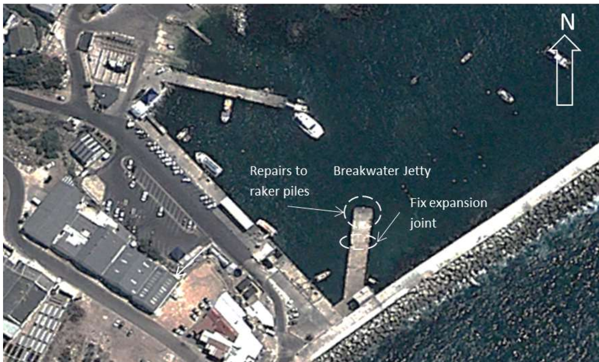
Figure 2-6: Breakwater Jetty Structure
