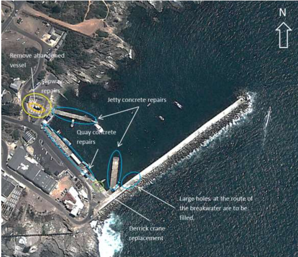
Figure 2-2: Work required in the Hermanus Harbour
