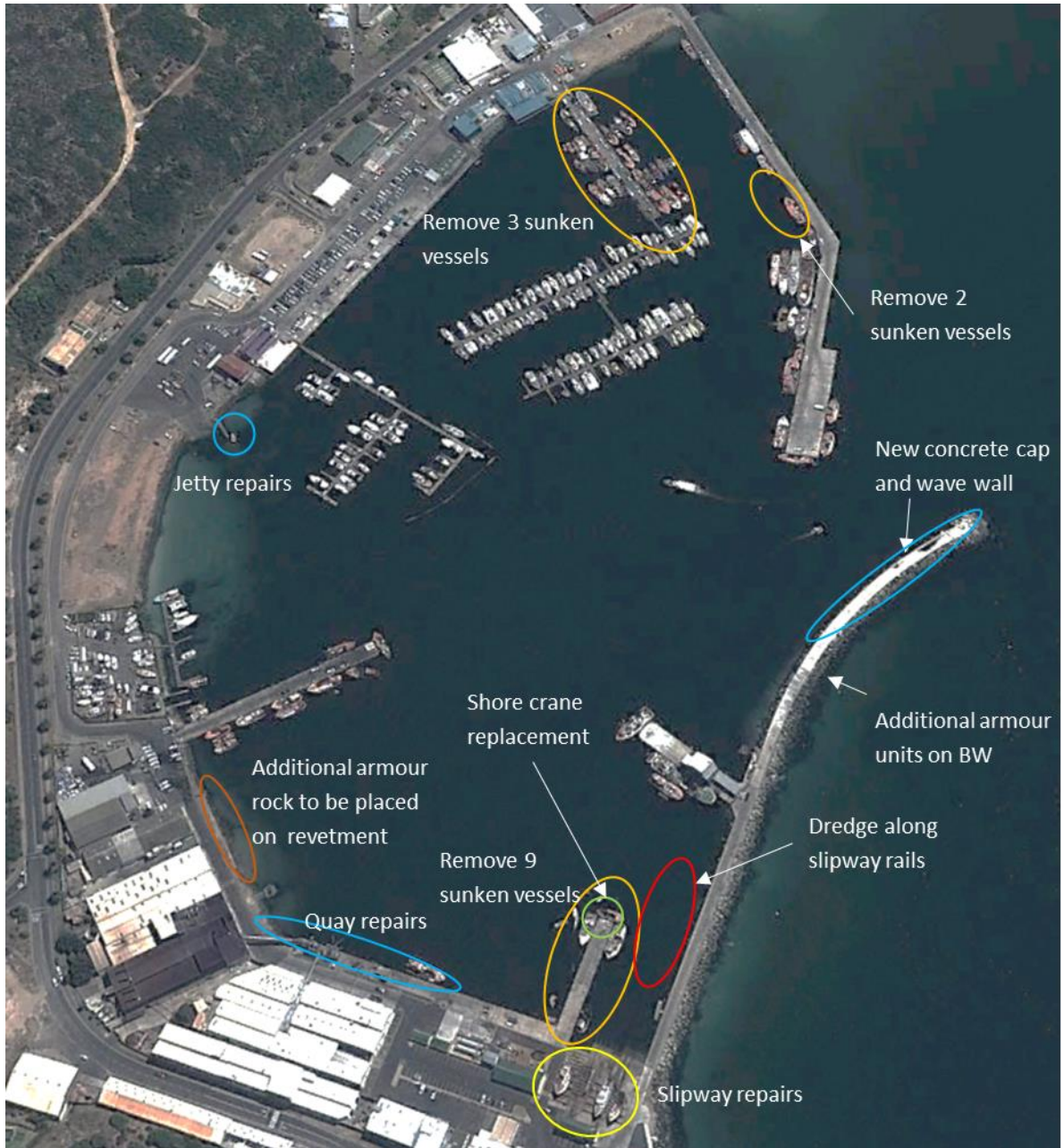
Figure 2-2: Work required in the Hout Bay Harbour
