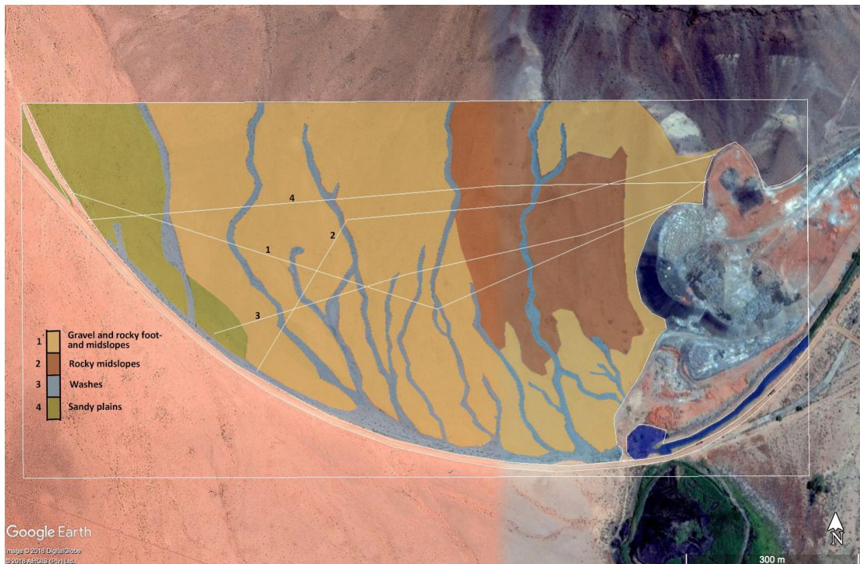
Figure 13. Vegetation map of the study site indicating communities 1 - 4. The selected route of the haul road (1) and the other screened-out alternatives (2, 3 & 4) are indicated with white lines.
