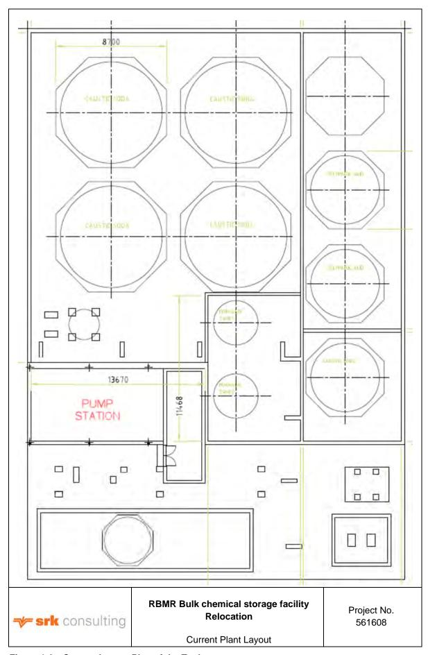
Figure 1-3: Current Layout Plan of the Tanks
