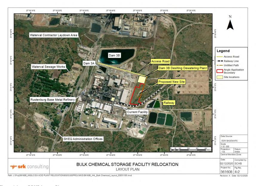
Figure 4-2: RBMR Layout Plan
