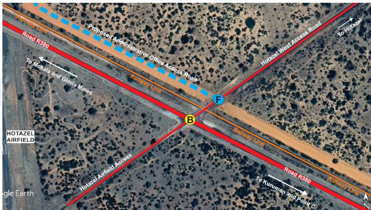
Figure 12-46: Proposed Kipling administrative office access from and to Hotazel west access road
