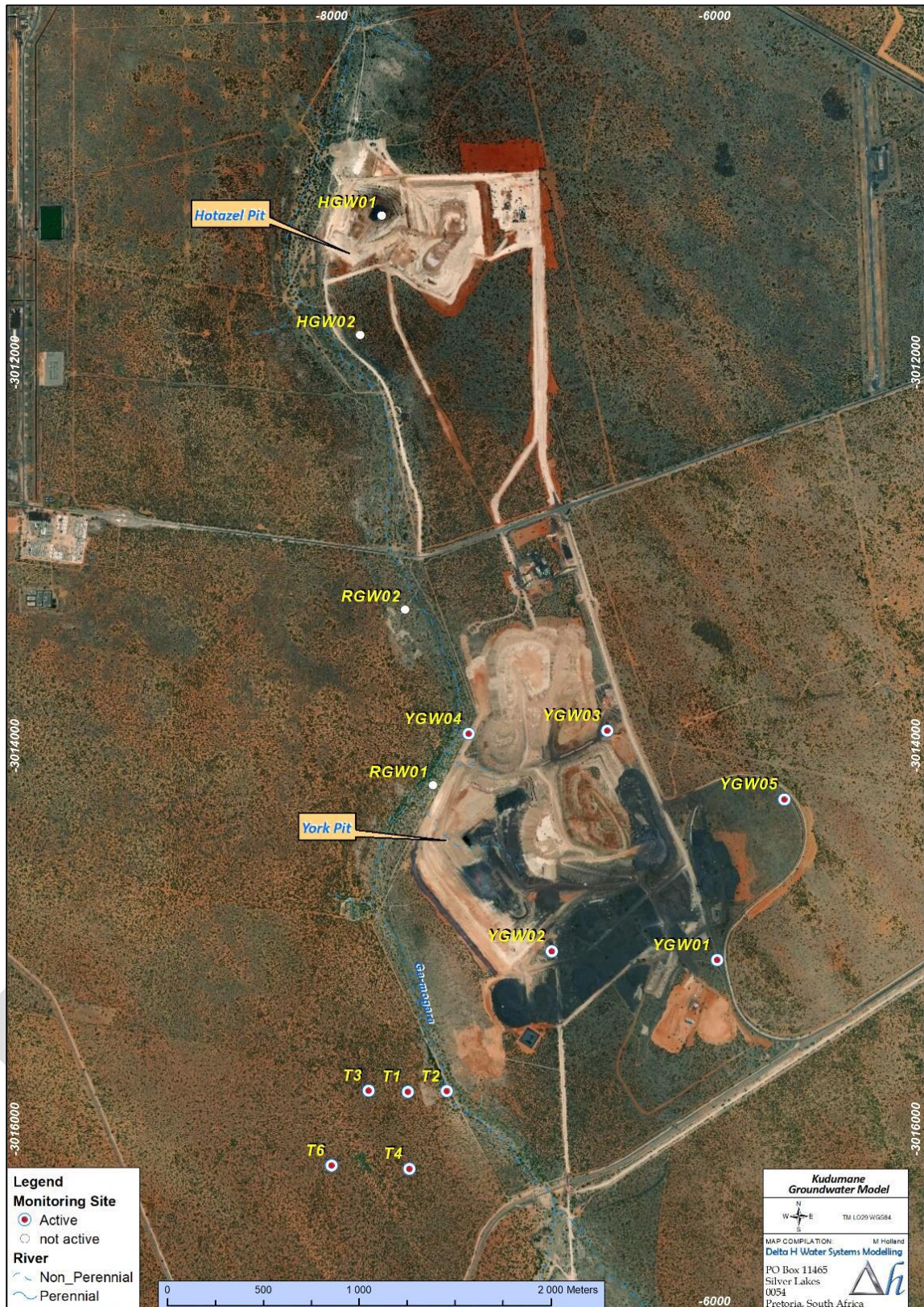
Figure 12-3: Location of the KMR groundwater monitoring boreholes in relation to the mine (DeltaH, 2021)
