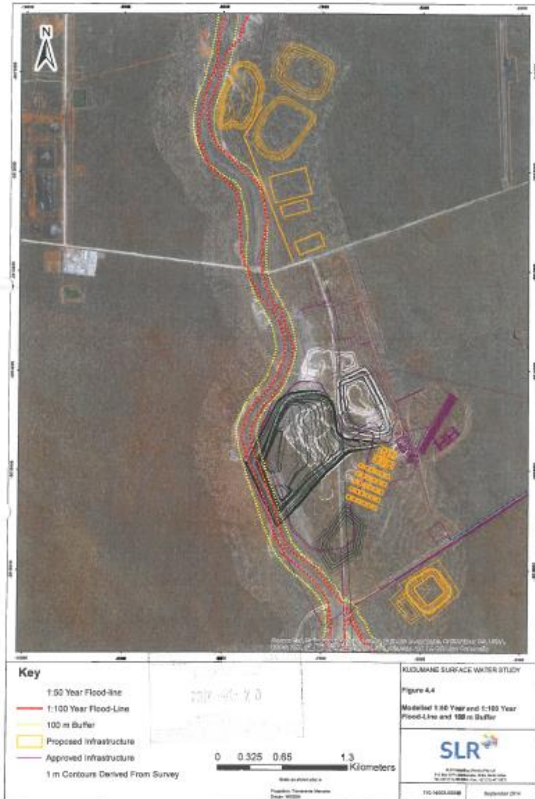
Figure 6-5. Modelled Floodline for 1:50 and 1:100 Storm Events (SLR, 2017)
