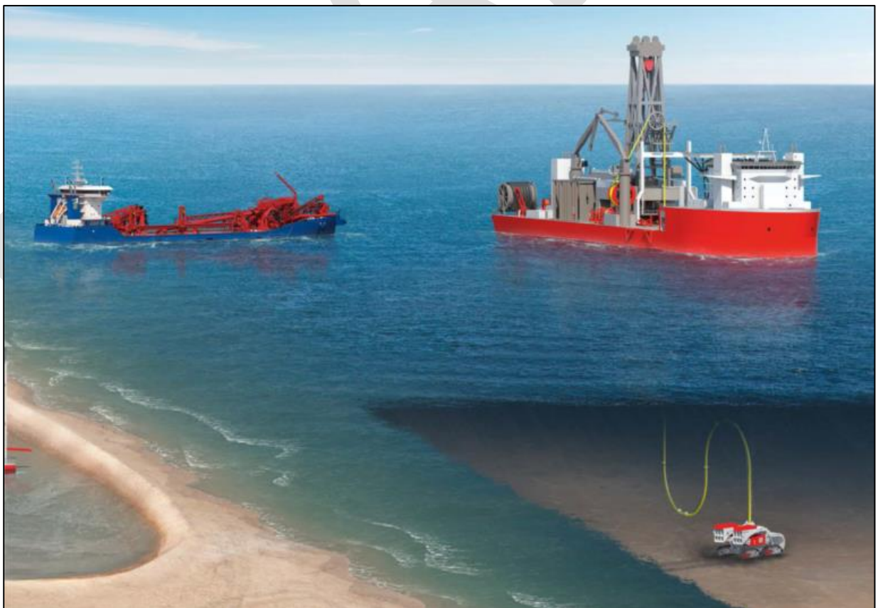
Figure 4-2: Schematic Representation of a Seabed Crawler in Operation ( https://waterkeeper.org/news/why-you-should-care-about-seabed-mining/ , 2023).
