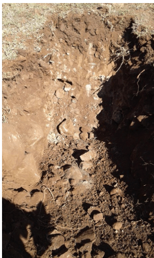
Plate 6: Typical profile of very soft to soft rock dolerite with hard rock corestones at Iphiva 6 (as observed in IP9)
