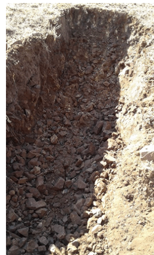
Plate 7: Typical profile of medium hard to hard rock dolerite at Iphiva 6 (as observed in IP8)
