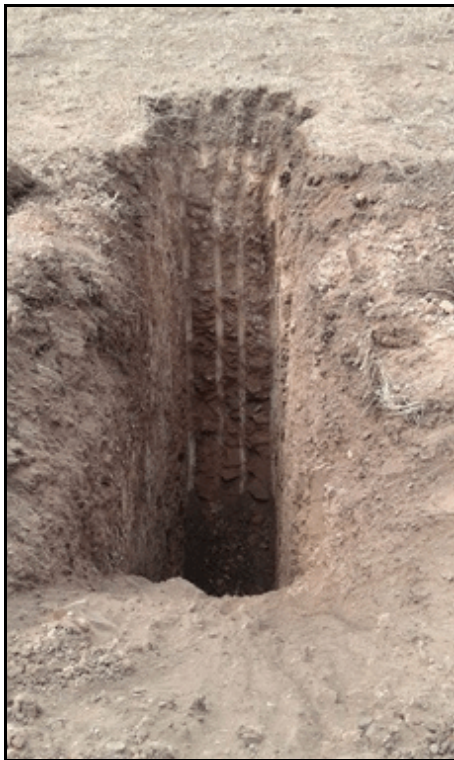
Plate 5: Typical subsoil profile of hillwash and residual basalt overlying basalt bedrock (IP1).
