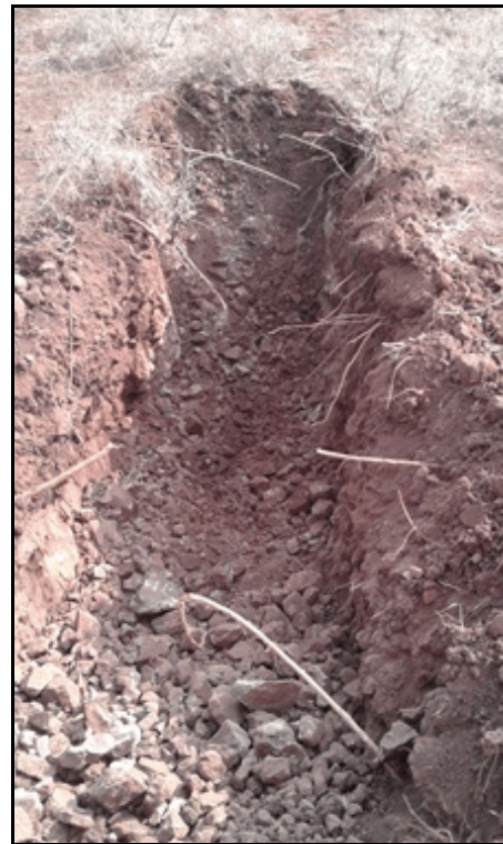
Plate 6: Typical shallow subsoil profile of hillwash directly overlying basalt bedrock (IP6).
