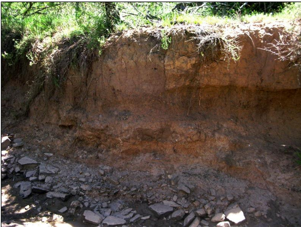
Figure 36. Riverbank section through semi-consolidated Quaternary to Holocene gravelly to sandy alluvium (Loc. 273).
