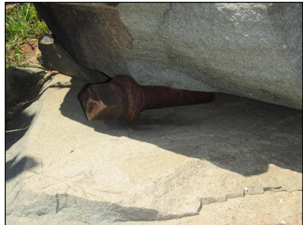
Figure 26: A metal rod that was hammered into a crack in the rock as part of the process of quarrying at waypoint 1748.
