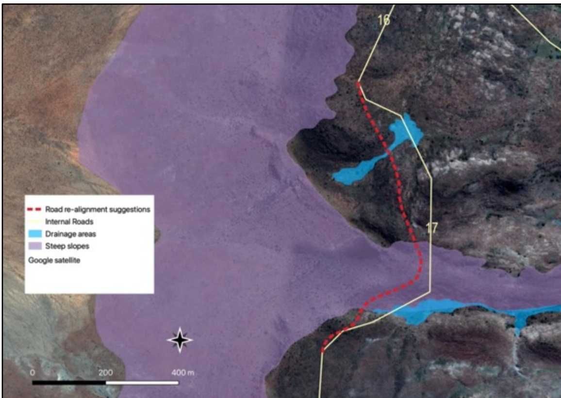
Figure 70: Proposed road layout between WTG16 and WTG18 - designed road in yellow, proposed change as dotted red lines.
