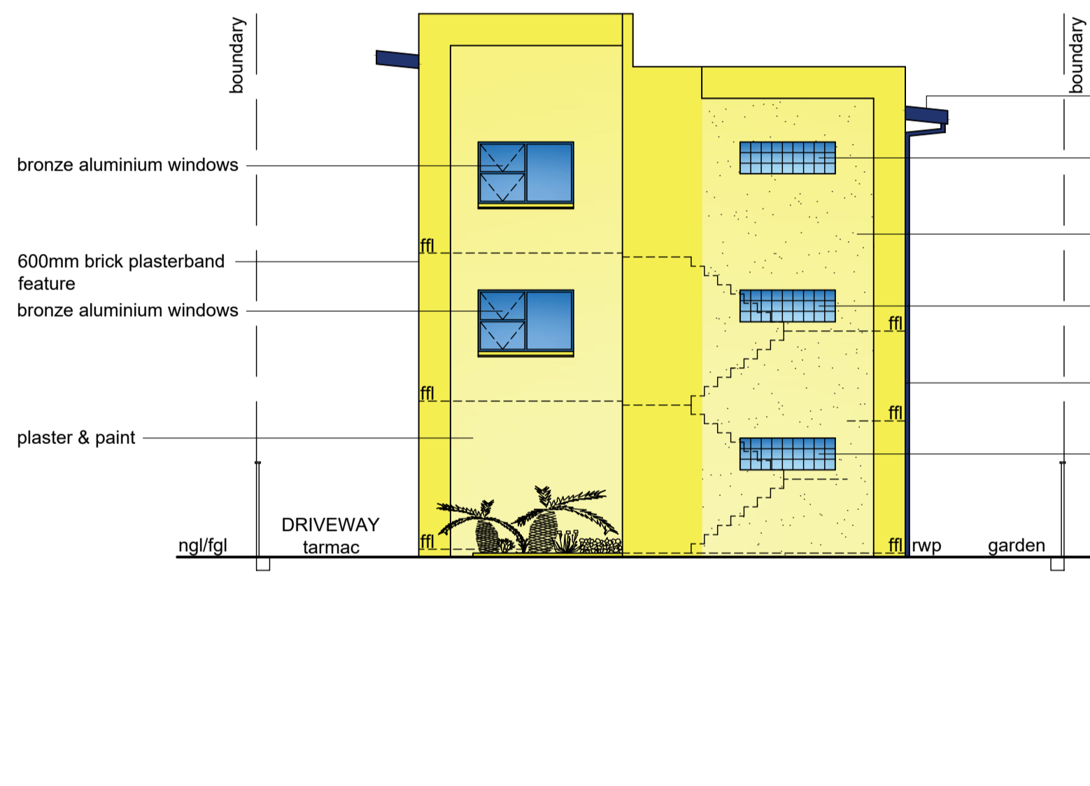
NORTH WEST ELEVATION
