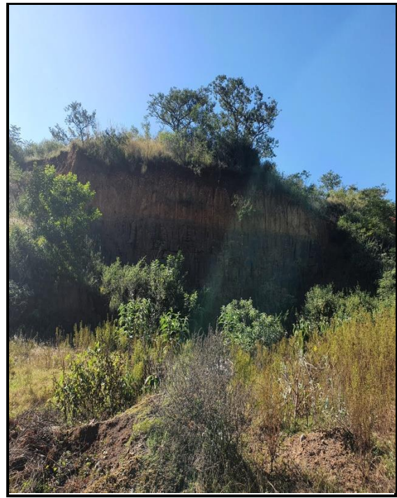
Plate 10: Indicative view of residual dolerite (top) and grey weathered shale rock at EXP1 (bottom)
