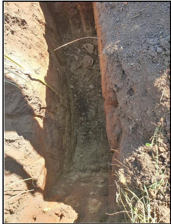
Plate 8: Indicative view of residual soils and weathered shale rock at IP13
