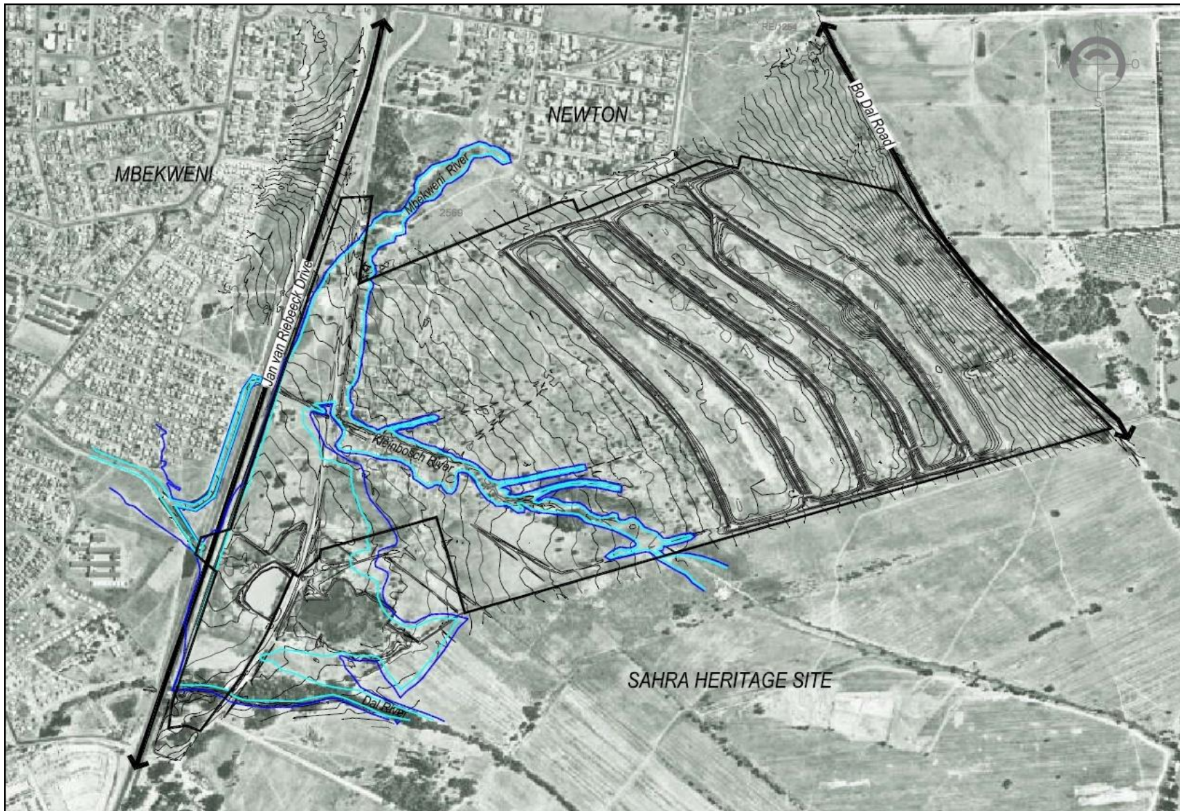
Figure 22: Topography and Drainage of the site
