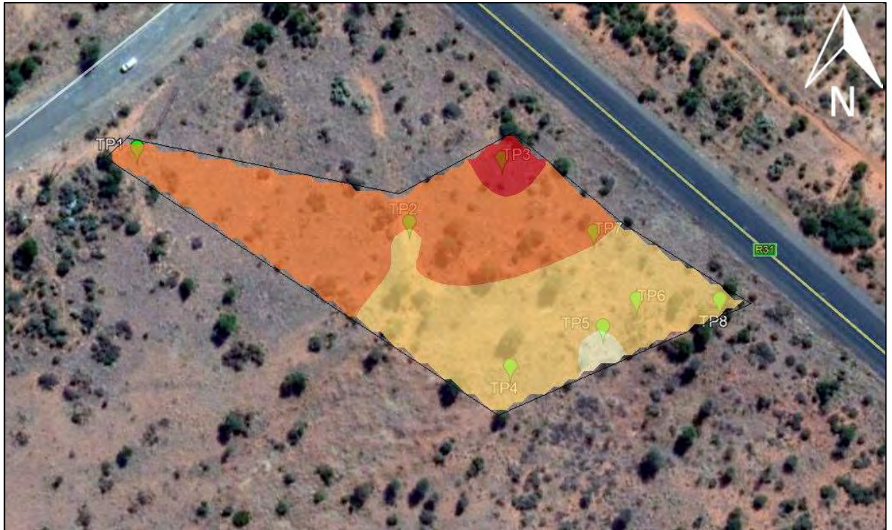
Figure 4 – Graphical illustration of Expected Refusal Depth
