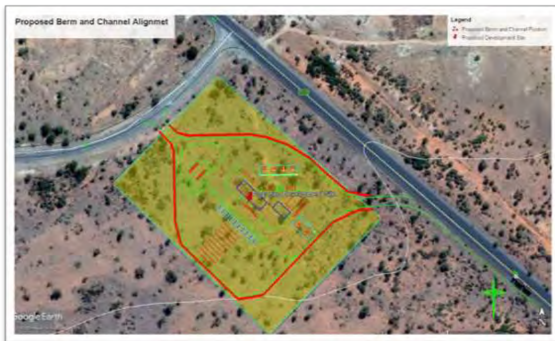
Figure 10: Proposed Berm and Channel Alignment
