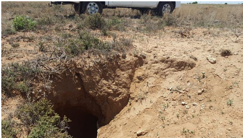
Figure 8.23: Photograph of typically occurring Gamoep soil form, with the hardpan carbonate just visible in the bottom right of the burrow excavation.
