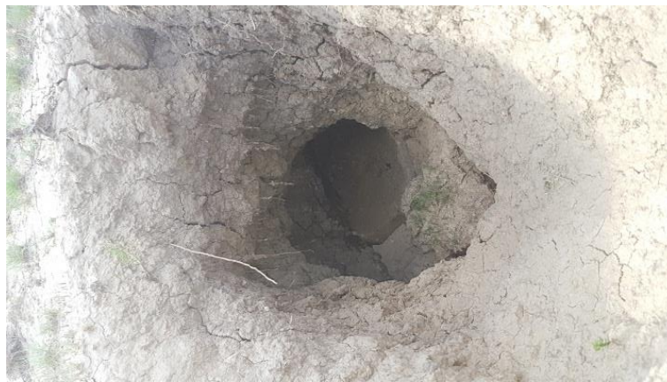
Figure 8.30: Photograph of Valsrivier soil profile from the study area, where shallow clay occurs in the subsoil.
