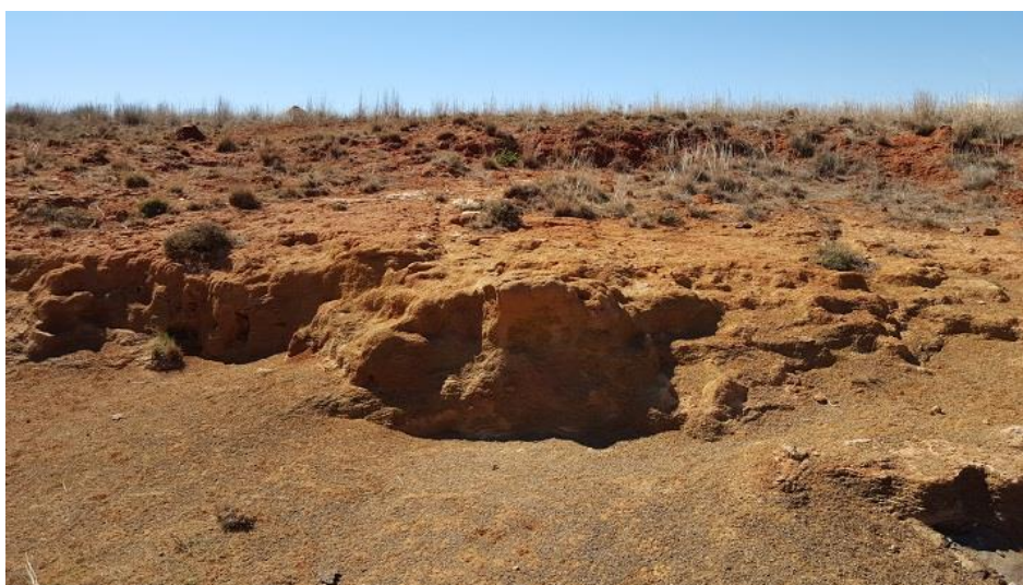
Figure 8.28: Photograph from an excavation in the study area of shallow Hutton soil on underlying dolerite.
