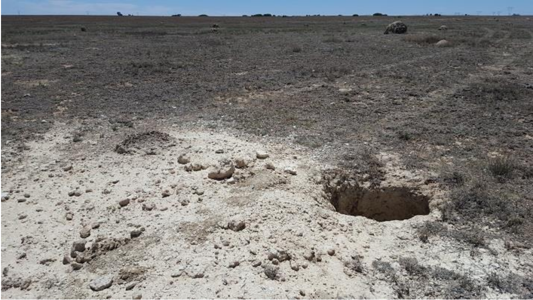
Figure 8.25: Photograph of Valsrivier soil profile from the site, where shallow clay occurs above a hardpan carbonate horizon.
