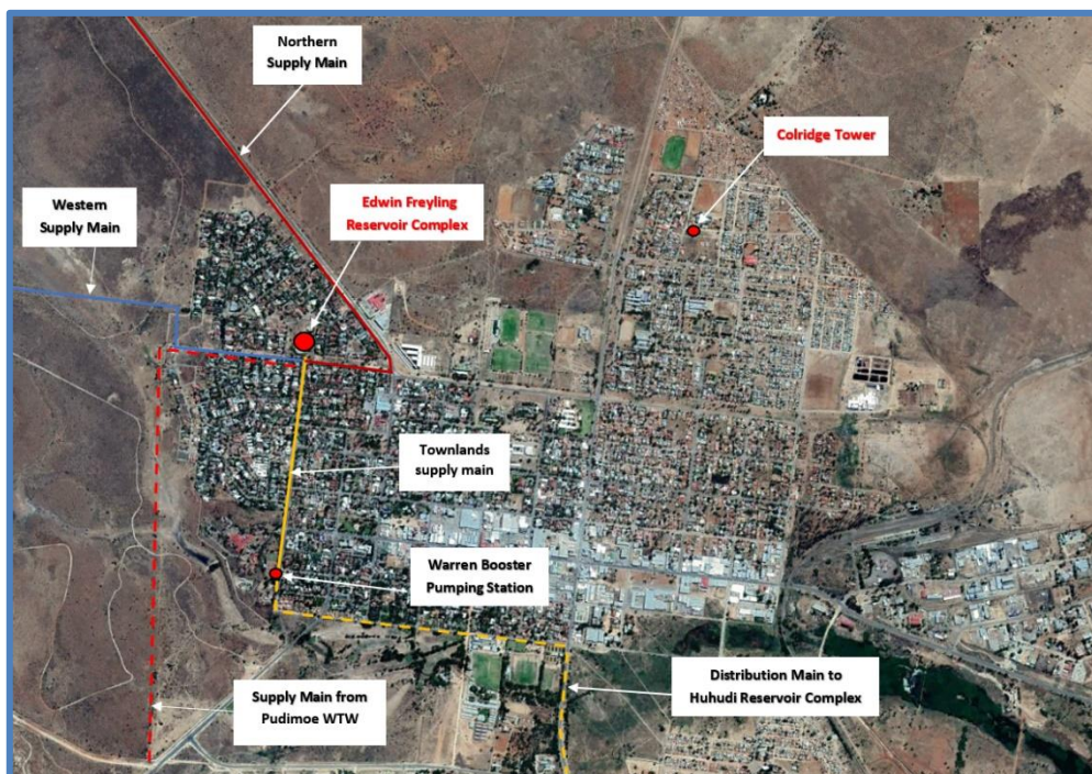
Figure 19: Existing Vryburg Water Infrastructure.
