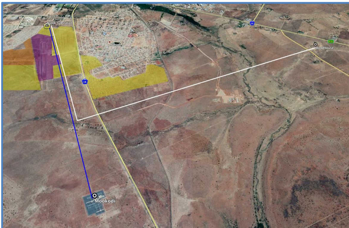
Figure 28: West Bulk Supply Proposal
