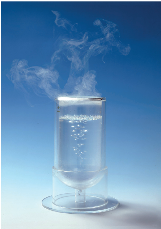
Figure 1. LNG “boiling” at atmospheric pressure and temperature (Source: OSAKA Gas)
