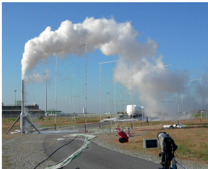
Figure 2. LNG Vapour Cloud created at ENGIE Lab CRIGEN LNG testing facility (Source: Engie Lab)
