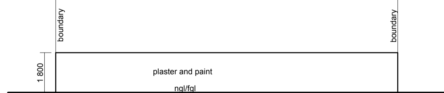
NORTH EAST ELEVATION - BOUNDARY WALL 2 - 1:00
