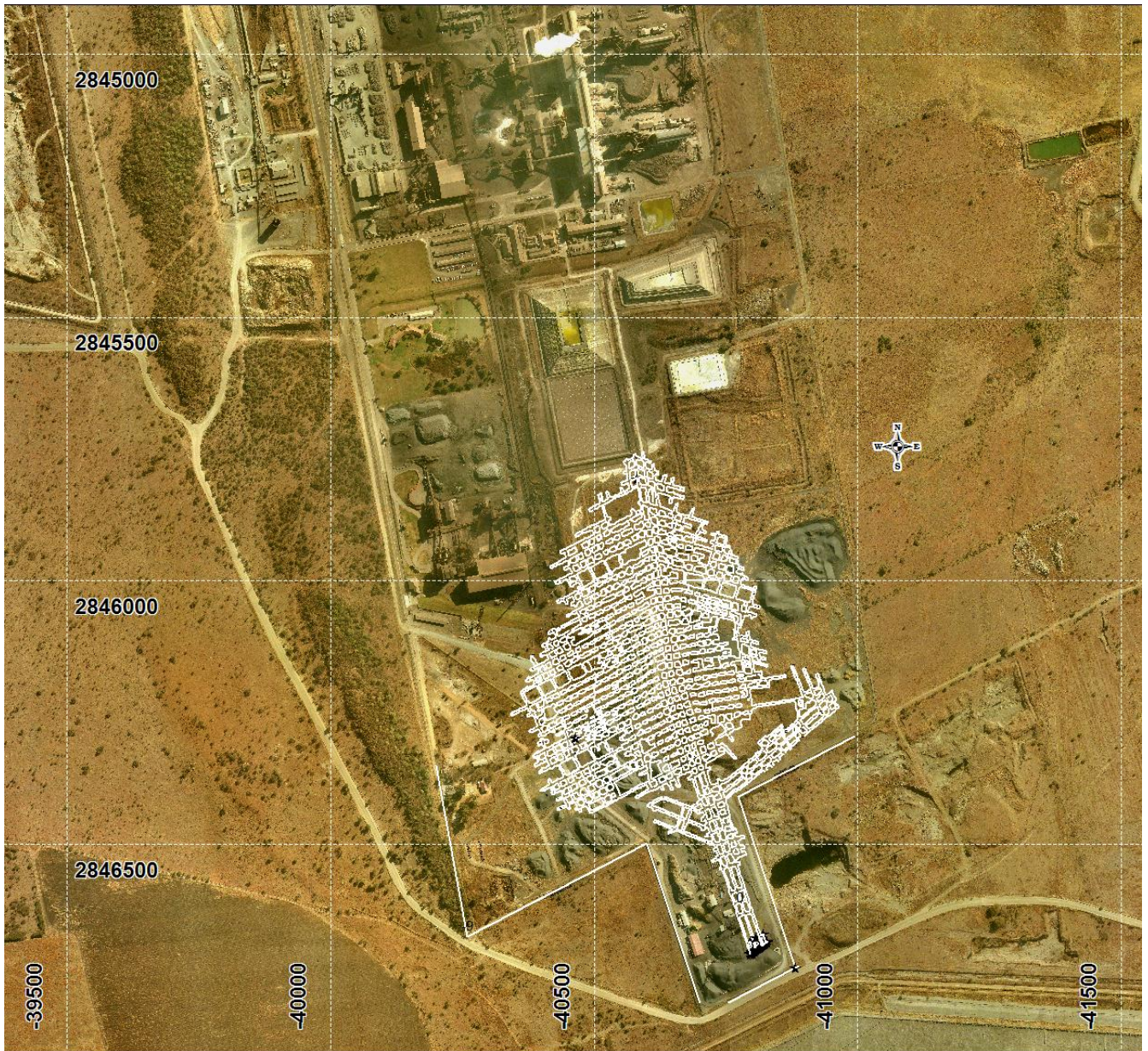
Figure 4(c): Mine Management Area (MA1) with the Underground Mine Layout.
