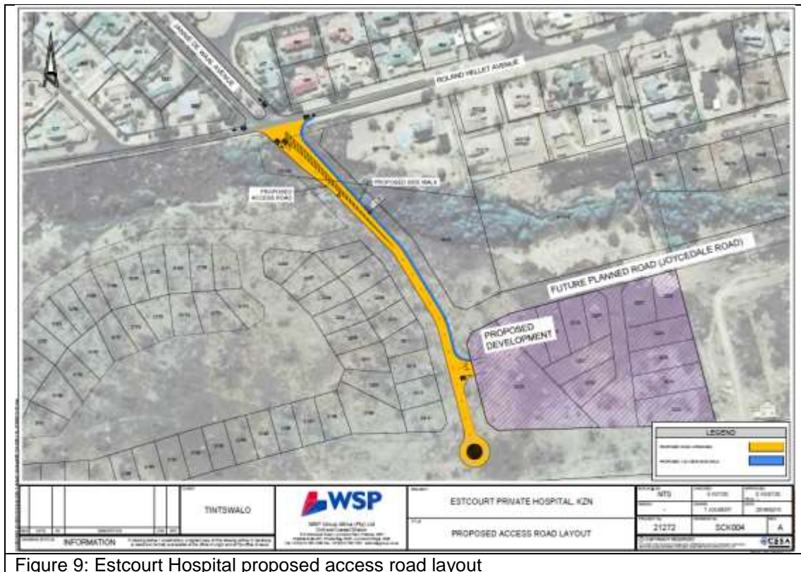
Figure 9: Estcourt Hospital proposed access road layout
